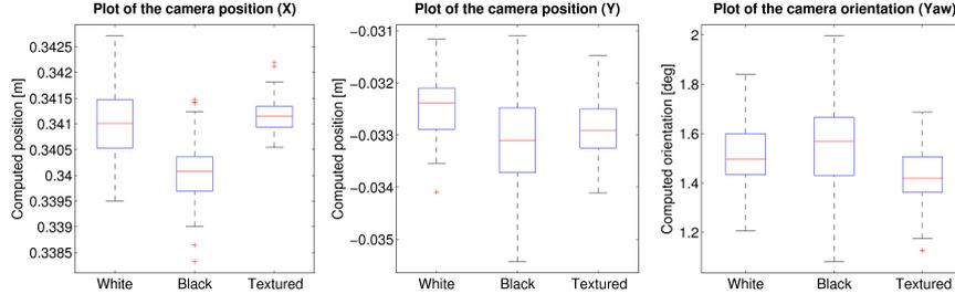
Fig. 7: Box diagram of the identified camera position (X/Y) and yaw angle (robot body frame).
