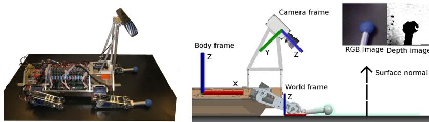
Fig. 1: Left: Picture of ALoF in the calibration configuration (the robot is placed on leveled ground with the front feet in the range of the RGB-D camera).
