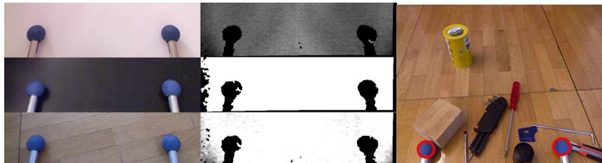
Fig. 5: Left side: Sample images of the different surfaces acquired from the RGB camera. Middle images: The corresponding depth images (the color has been normalized for visualization). Right side: Sample image of the foot detection in a disturbed scene.
