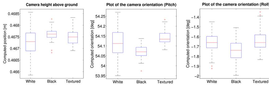
Fig. 6: Box diagram of the identified camera height above ground as well as pitch and roll angle.
