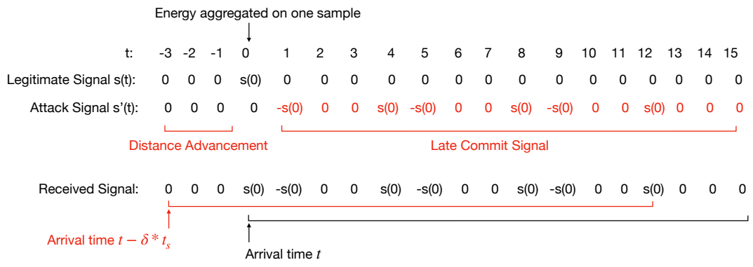
Figure 21: An example of the ED/LC attack on the V-Range symbol when a receiver performs FFT for data detection.
