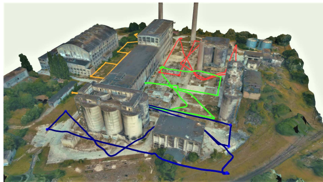
Fig. 1: 3D-view of the proposed system guiding safe and successful navigation of a team of four UAV-agents (with trajectories shown in different colors) in a photo-realistic simulation of an industrial site, despite that the user-defined waypoints for the UAVs correspond to partially overlapping regions. Via hierarchical planning, the proposed system is able to safely plan the UAVs’ paths, running state estimation and local obstacle avoidance onboard each UAV, and sensor fusion and multi-robot global planning on the server to collect all UAVs’ experiences in a joint, optimized map.
