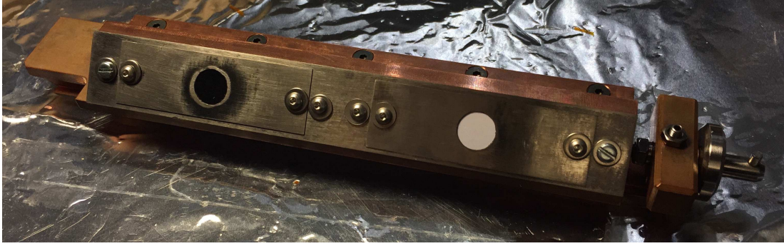
Figure 4.24: Picture of thin Ti foil TANDEM proton irradiation mount mainly fabricated out of \sim 300 g copper to ensure a good heat dissipation. The copper parts are protected from irradiation by a 0.3 mm thick W beam dump. The thin Ti foil (black, on the left) is held by another W baffle. A piece of paper on the right is mounted for calibration purposes of the proton beam.
