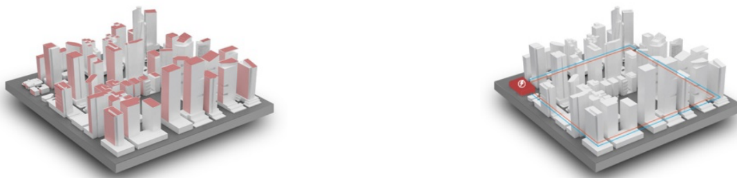
Figure 4: Schematic presentation of cooling systems' location (in red) in decentralized (left) and centralized (right) buildings in the study area.
