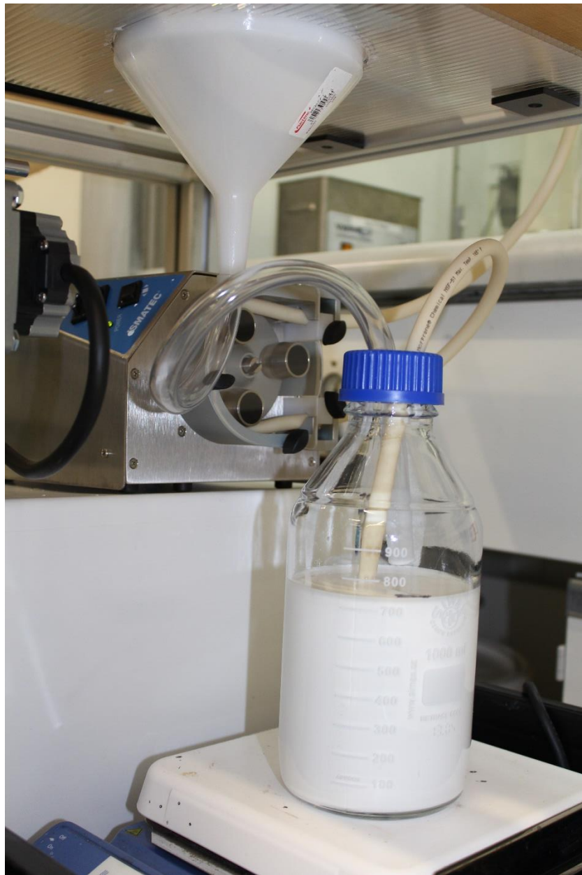
Slurry reservoir for continuous curtain operation. During deposition the slurry is agitated by a magnetic stirrer.
