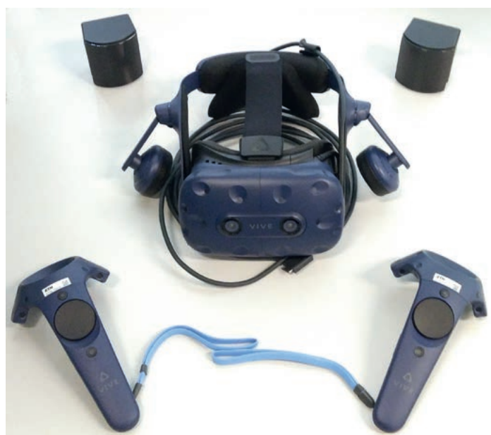
Fig. 1. A virtual reality device (here: 'Vive Pro' from HTC) consisting of a headset (center), two hand-held control sticks (bottom left and right) as well as two base stations used to track a person's position (top left and right).
