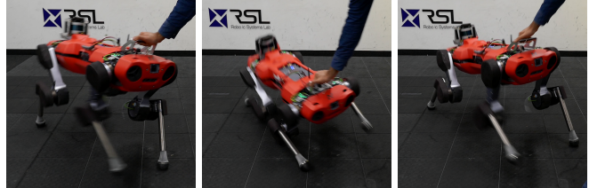
Fig. 1. ANYmal being pushed around while running a learned policy.
