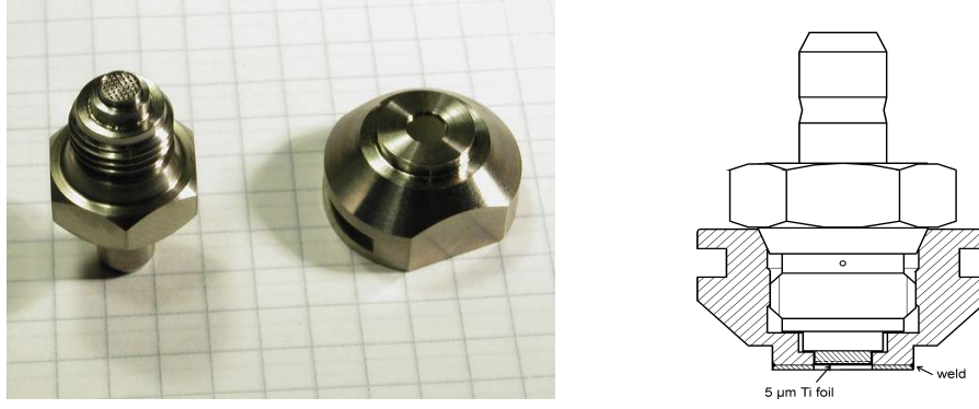
Figure 11: Picture (left) and drawing of ^{22}\text{Na} source capsule ( from : [91])
