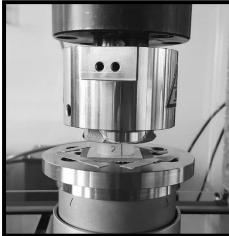
Figure 5-3: Mechanical testing set-up for disc models. The samples were put between Parafilm and sandpaper on each side to ensure some friction but prevent soaking of the sandpaper.
