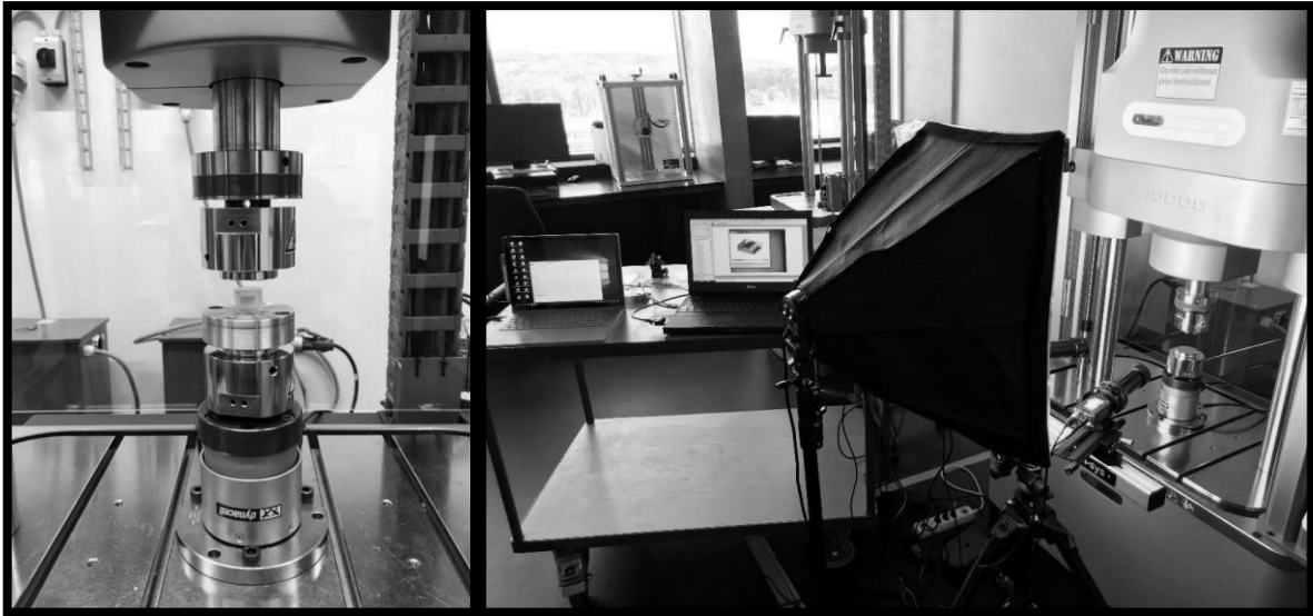
Figure 5-4: Setup of the INSTRON E10000 machine and the setup of the VIC 3D image correlation system.
