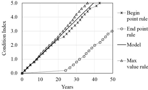
Figure 5 Alternative assignment rules; adding uncertain rates of deterioration.
