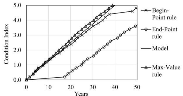
Figure 4 Non-Parametric deterioration curves using alternative assignment rules
