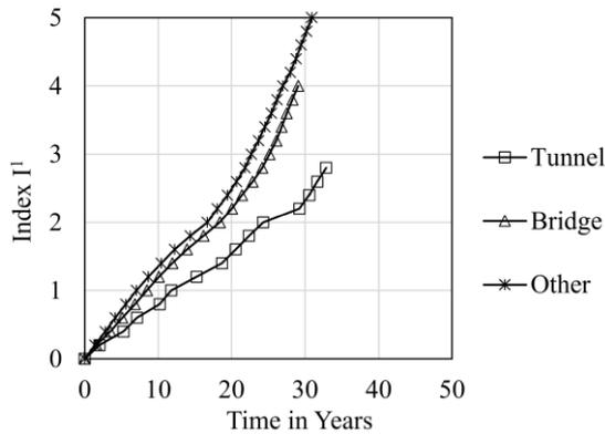
Figure 10 Deterioration curves for tunnels, bridges and other
