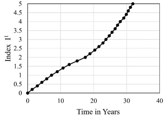
Figure 1 Example of a non-parametric deterioration curve
