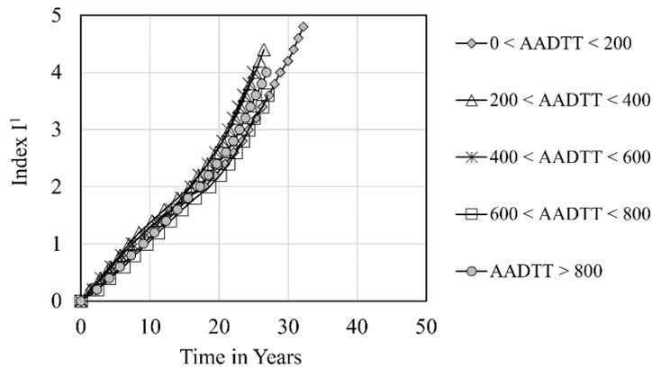
Figure 9 Non-Parametric deterioration curves of general surface damage
