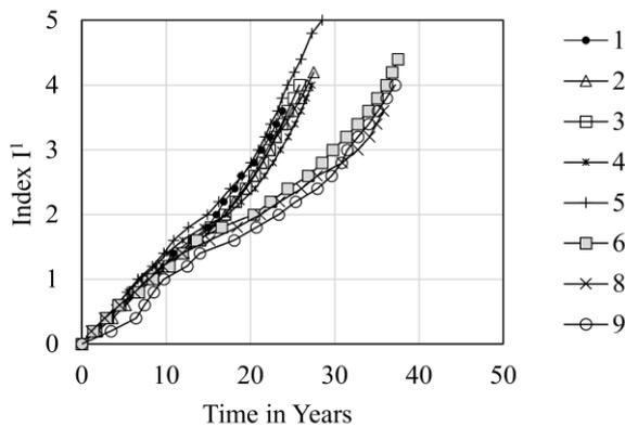
Figure 12 Non-Parametric deterioration curves using a combined index of climate and axle load as difficulty factors.
