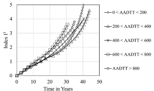
Figure 8 Non-Parametric deterioration curves of rutting
