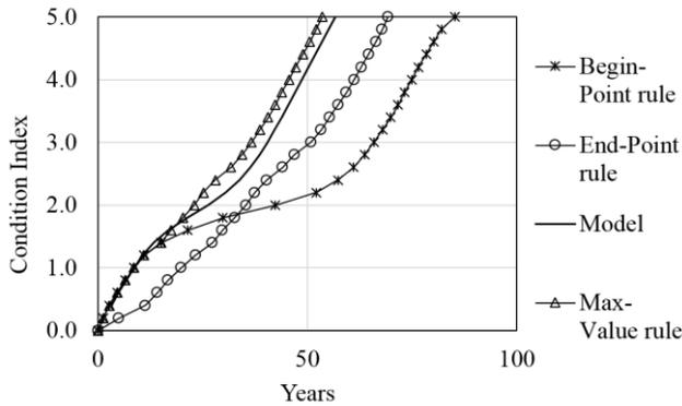
Figure 7 Alternative assignment rules; adding an S-shaped deterioration curve and a larger sample size
