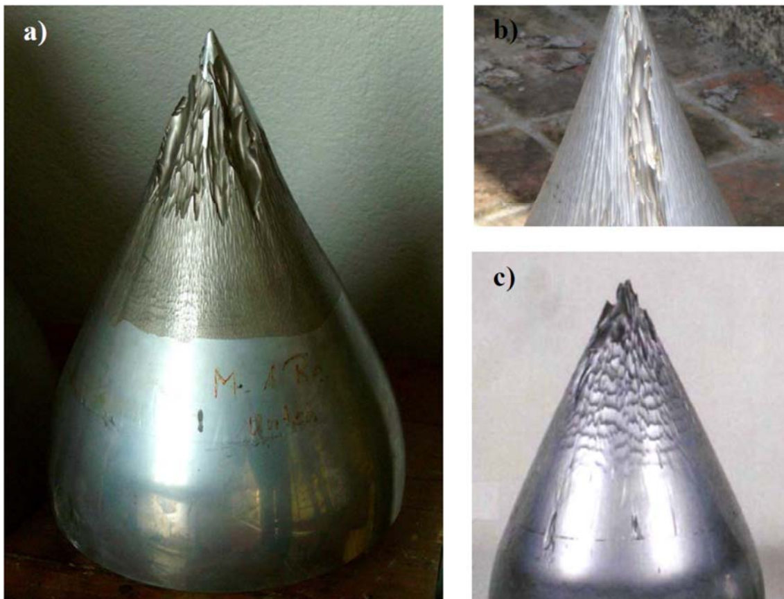
Figure 2-10 Eroded uncoated needle tips of Pelton turbines a) HPP Rabiusa-Realta, Switzerland (courtesy A. Abgottspon), b) Chilime HPP, Nepal (Bajracharya et al. 2008), and c) example reported by Cateni et al. (2008) / Hamerak (2016).
