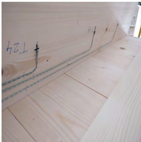
Figure 4.7: Wire thermocouples of CLT ( 0.5 \text{ mm}^2 conductor area) attached to lamellae before the bonding process in a hydraulic press. Own image.
