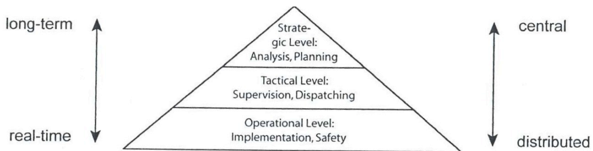
Figure 1 Functional structure of public transport operations and planning
