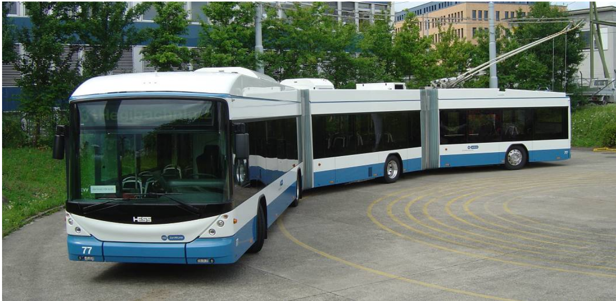
Figure 16 Double articulated trolley buses providing service in Line 31
