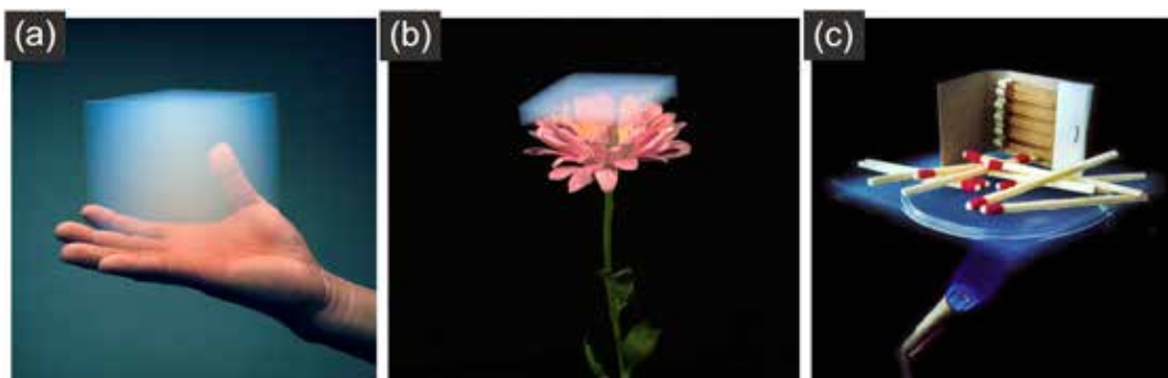
Fig. 5. Photographs of silica aerogels showing exceptional properties such as light weight and low thermal conductivity. The bluish haze, aerogels are often referred to as ‘frozen smoke’, is the result of Rayleigh scattering (Credit: (a, c) Courtesy NASA/JPL-Caltech, (b) Laboratory for Multifunctional Materials, ETH Zürich).
