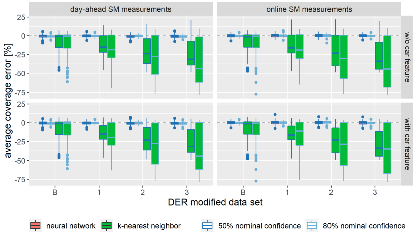
FIGURE 9.14: Average coverage error of the quantile forecasts of active power flow for all lines and time steps in the test set. Prediction intervals with 50% and 80% nominal confidence are considered. 5
