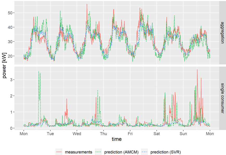
FIGURE 9.2: Measurements and associated predictions based on the AMCM and SVR algorithms for two representative load profiles.
