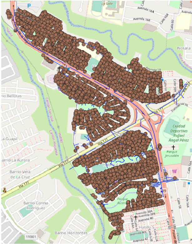
FIGURE 3.6: Illustration of a digitized section with corresponding loads from the distribution network of the City of San José operated by CNFL.
