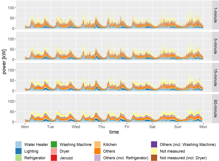
FIGURE 5.5: Load profiling of the aggregation of 70 residential users displayed at different temporal resolutions.
