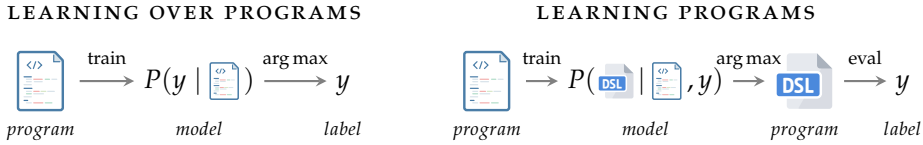
FIGURE 1.1: High-level illustration of two perspectives considered in our work that learn to predict program properties from a dataset of programs. Learning over programs directly learns a machine learning model that predicts a given property. In contrast, learning programs learns a program from a domain-specific language which, when evaluated, computes the property.
