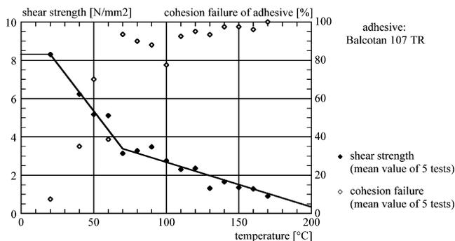
**Fig. 3** Mean shear strength and percentage of cohesion failure observed for the adhesive Balcotan 107 TR as a function of temperature
