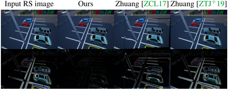
Figure 6.7.: Qualitative comparisons against state-of-the-art methods on the Carla-RS dataset. Second row: Residual image, which is defined as the absolute difference between the corresponding image and the ground truth global shutter image I_{gt}^g .
