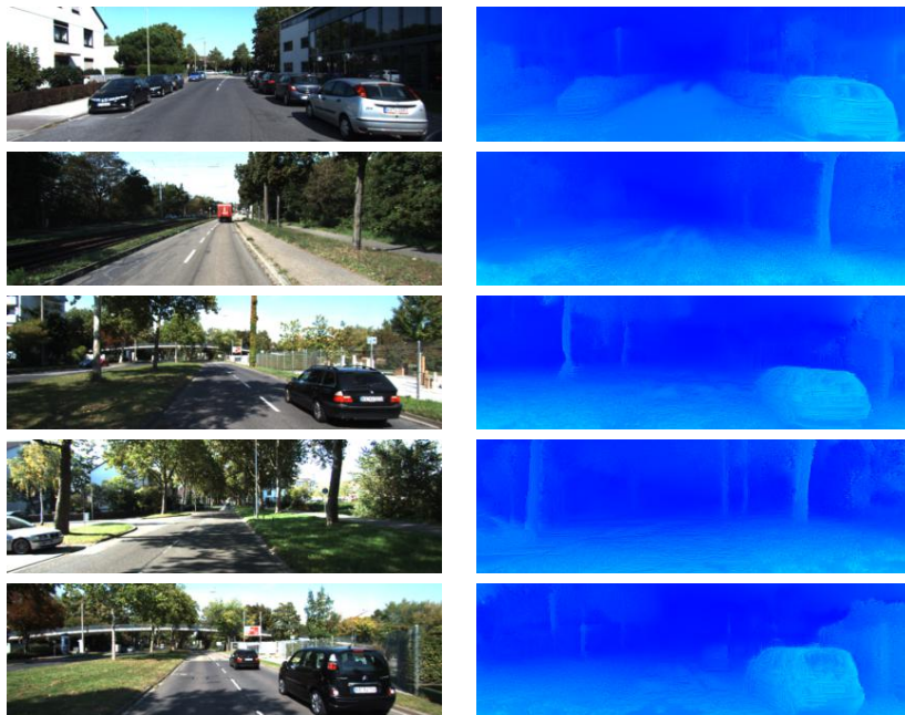
Figure 8.2.: Single image depth prediction of our sinSfM network. Left: Input test image. Right: Predicted depth map of our trained depth network. It demonstrates that our depth network is able to predict reasonable depth maps, even trained with a single frame motion estimation network.
