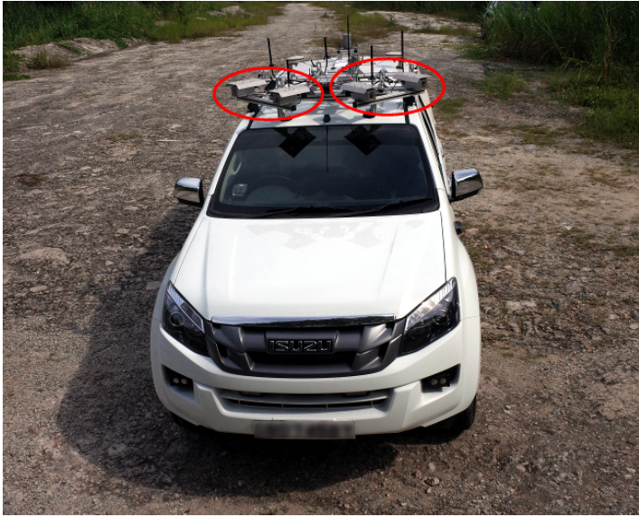
Figure 3.2.: Isuzu D-Max platform equipped with two fisheye-stereo cameras which are shown enclosed in red ellipses.
