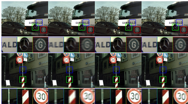
Figure 5.5.: Qualitative comparisons on synthetic dataset. First: Ground truth sharp image. Second: Input blurry image. Third: Deblurring results of the supervised method from Tao et al. [TGS + 18]; The network is retrained on our dataset. Fourth: Deblurring results of the proposed self-supervised learning method.
