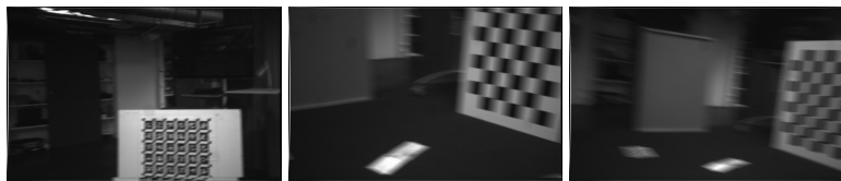
Figure 7.5.: Examples images from the proposed dataset for benchmarking visual odometry from motion blurred image sequences. The dataset contains multiple sequences with varying levels of motion blur.
