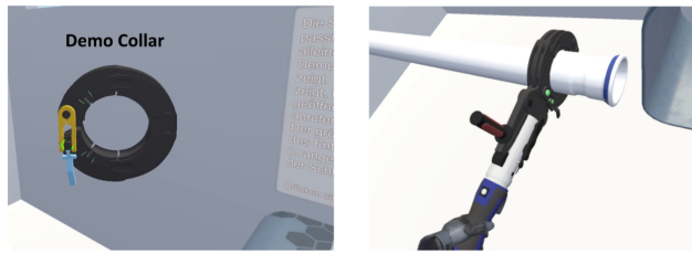
Figure 2: Objects in the VTE. Left: Enlarged version of the collar; Right: Pressing tool attached to pressing collar on pressfitting.
