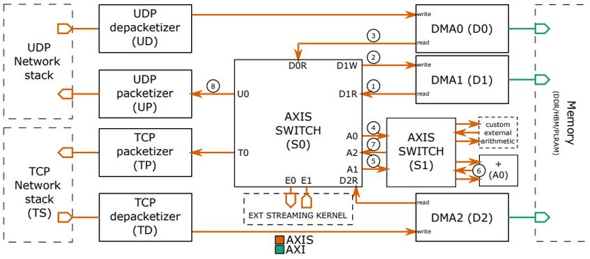
Fig. 2: Schematic view of CCL Offload Data plane and datapaths.
