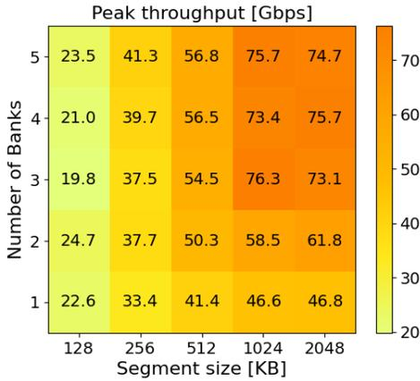
Fig. 5: Effect of segmentation and channels on throughput.
