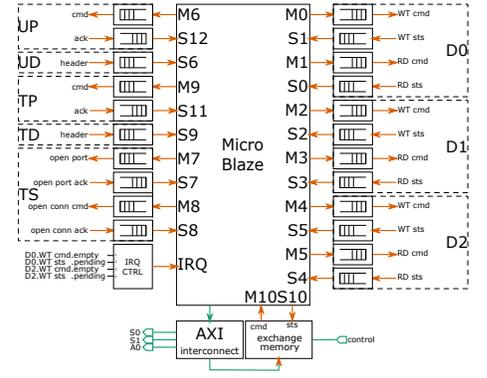
Fig. 3: Schematic view of CCL Offload Control plane.
