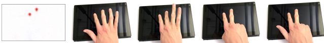
Figure 7: The same capacitive image (left) can result from different hand poses due to variation in orientation of fingers not touching the screen. Here, Index and Middle are touching the screen.
