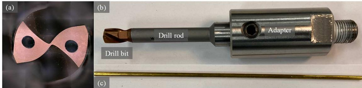
Fig. 2: (a) Top view of drill bit showing cooling channels; (b) Drilling tool configuration with adapter; (c) Connecting tube
