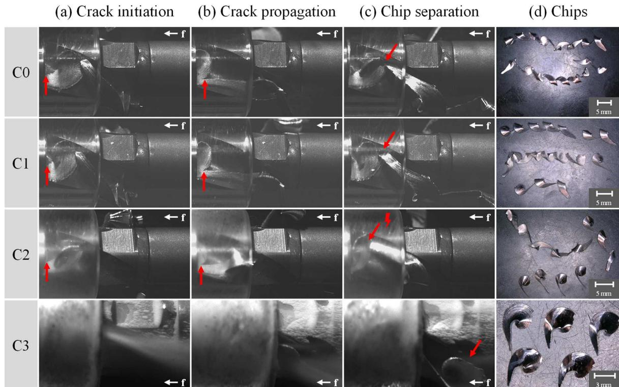
Fig. 4: Representative time steps of the chip formation and transport processes for C0, C1, C2 and C3: (a) Crack initiation, (b) crack propagation, (c) chip separation shortly before new crack initiation; (d) illustrations of representative Al-chips
