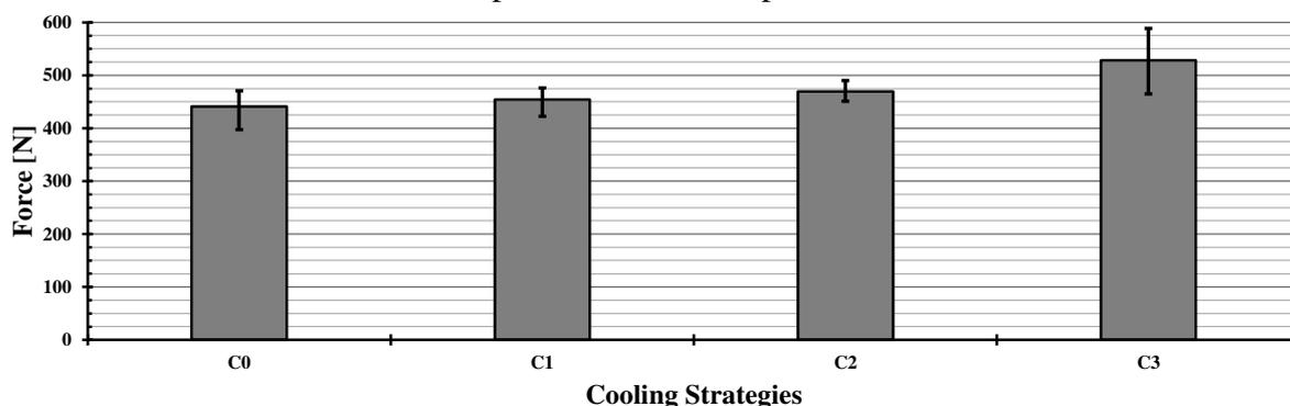
Fig. 5: Thrust forces for different cooling strategies C0, C1, C2 and C3
