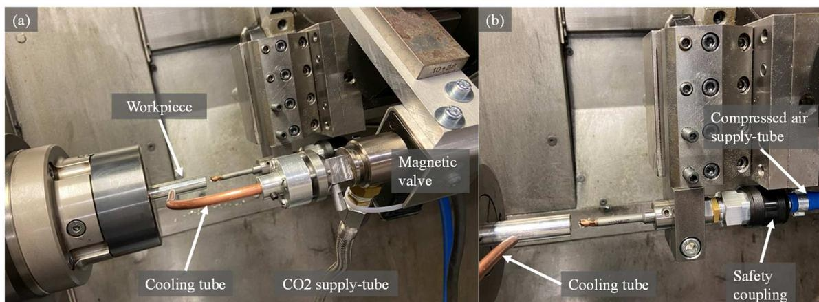
Fig. 3: (a) C2 cooling configuration showing the cooling from the CO<sub>2</sub> supply-tube to the magnetic valve through the cooling tube to the workpiece surface; (b) Combination of workpiece side cooling via cooling tube (C2) and tool-side cooling via compressed air supply tube (C1)
