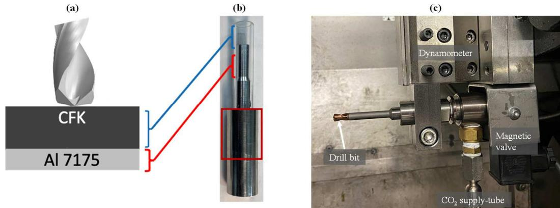
Fig. 1: (a) CFRP/Al-stack drilling illustration; (b) Sample to approximate an arbitrary stack-drilling process (CFRP entry, Al exit) made out of aluminium with PMMA tube highlighting workpiece side cooling area with red rectangle; (c) Test rig configuration for tool-side cryogenic CO<sub>2</sub> cooling with drill bit (C3)
