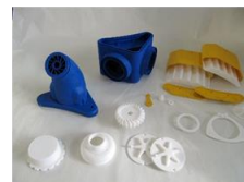
Laser powder bed fusion of plastics
