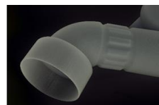
Laser powder bed fusion of plastics
