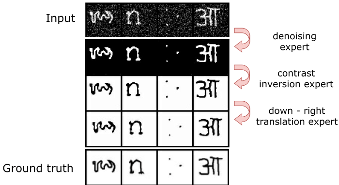
Figure 8: First row: input Omniglot letters that were transformed with noise, contrast inversion and translation up left. Second to fourth row: application of denoising, contrast inverting and right down translating experts. Last row: ground truth. Although the experts were not trained on a combination of mechanisms nor on Omniglot letters, they can be used to recover the original digits.
