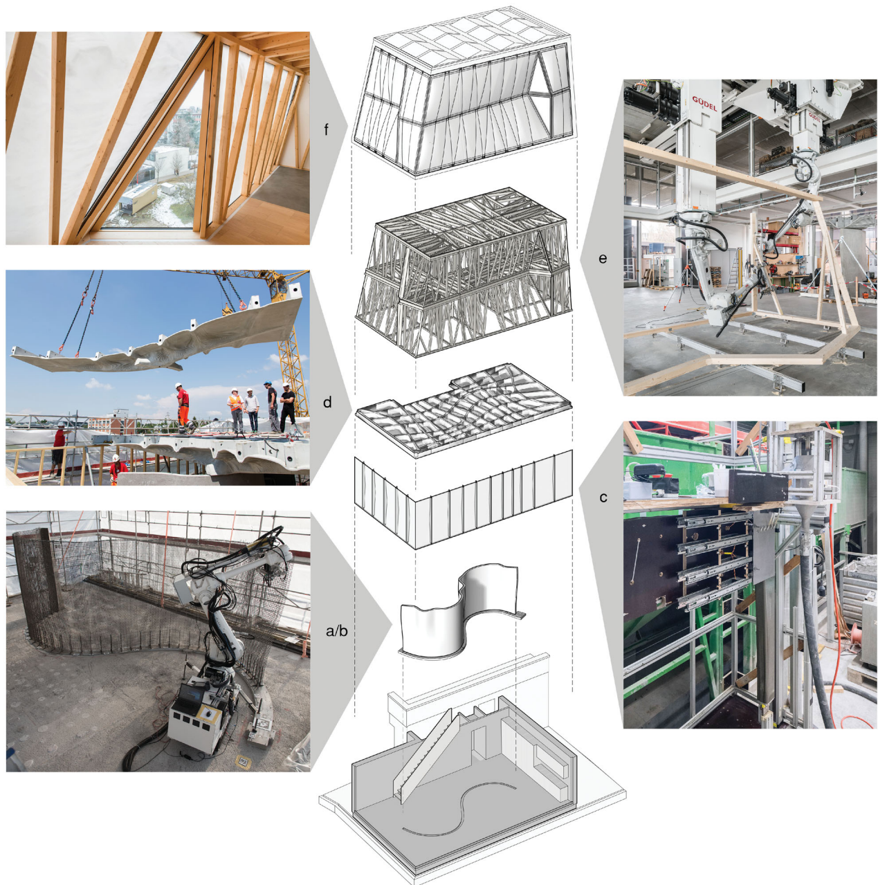
Figure 2. Building parts of DFAB HOUSE and associated DFAB applications: Mesh Mould (a), In Situ Fabricator (b), Smart Dynamic Casting (c), Smart Slab (d), Spatial Timber Assemblies (e), Lightweight Translucent Façade (f).
