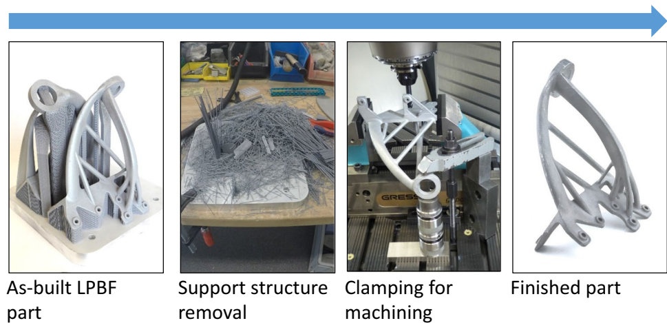
Fig. 1 Conventional LPBF post-processing chain highlighting the problematic removal of support structures and the required part clamping for machining
