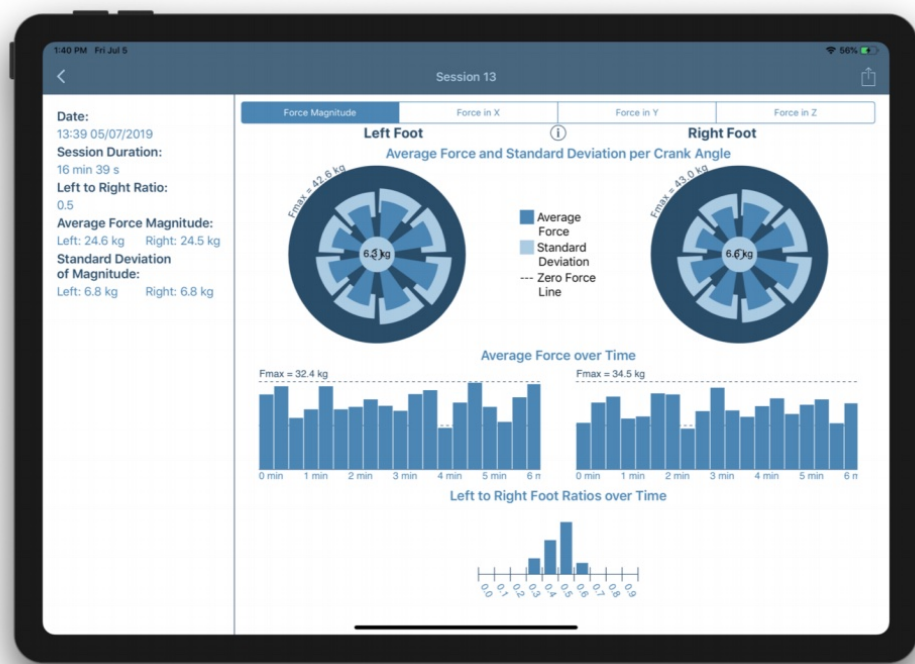
Figure 11. Pedalling forces breakdown. Post-session analysis showing breakdown of forces for different crank angles.
