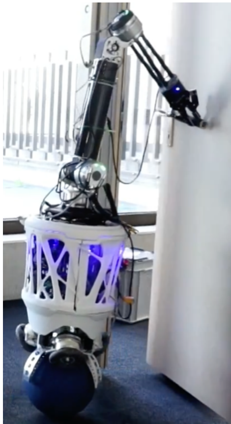
Figure 1.1: The ballbot with the 4-DOF DynaArm and a Robotiq-2F-85 gripper
