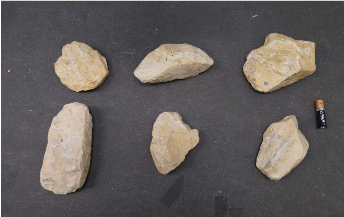
Figure 6.5: Limestones with irregular shape are used to create the vertical stacks.
