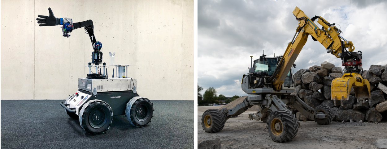
Figure 1.2: The work presented in this thesis has been mainly evaluated on the mobile manipulation platforms mANYpulator (left) and HEAP (right). Although varying in size considerably, they both are designed for a versatile interaction tasks and include complete onboard sensing and a force-controllable arm.
