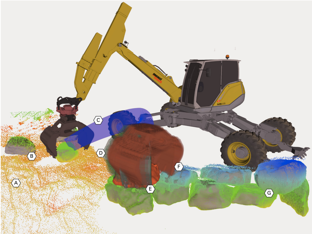
Figure 7.7: Grasp planning and placement of a stone to its desired location (red): (A) Collision and localization point cloud, (B) Stones localized in point cloud, (C) Spline motion trajectory, (D, Green) Collision free grasp hypotheses, (F, Red) Grasp hypotheses with collisions, (E) Selected grasp configuration, (G) The collision point cloud is augmented with point clouds of already localized stones.
