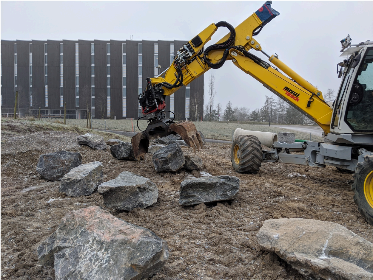
Figure 7.3: Initial state of stones, loosely distributed on the terrain. LiDAR mapping and RANSAC ground segmentation allows for initial detection and grasping for refined scanning in the gripper.
