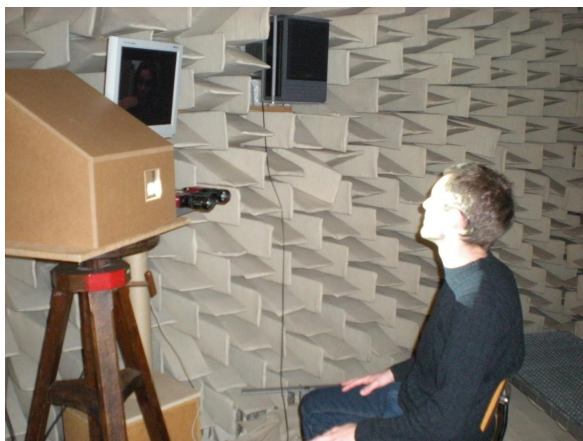
Figure 4.1: Recording setup: one speaker sits in front of the 3D scanner in the anechoic room while watching one of the eliciting videos clips.
