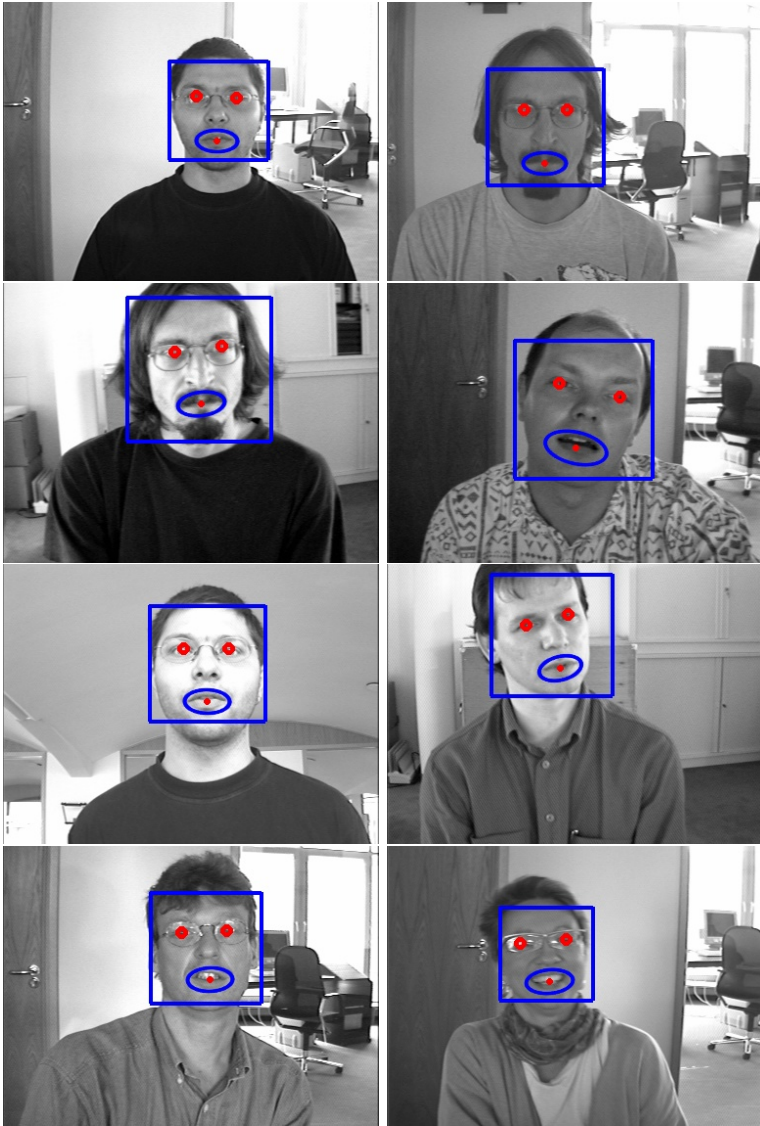
Figure 2.8: Some example successes of the system. Difficult situations like reflections on the glasses, facial hair and head pose changes are handled.
