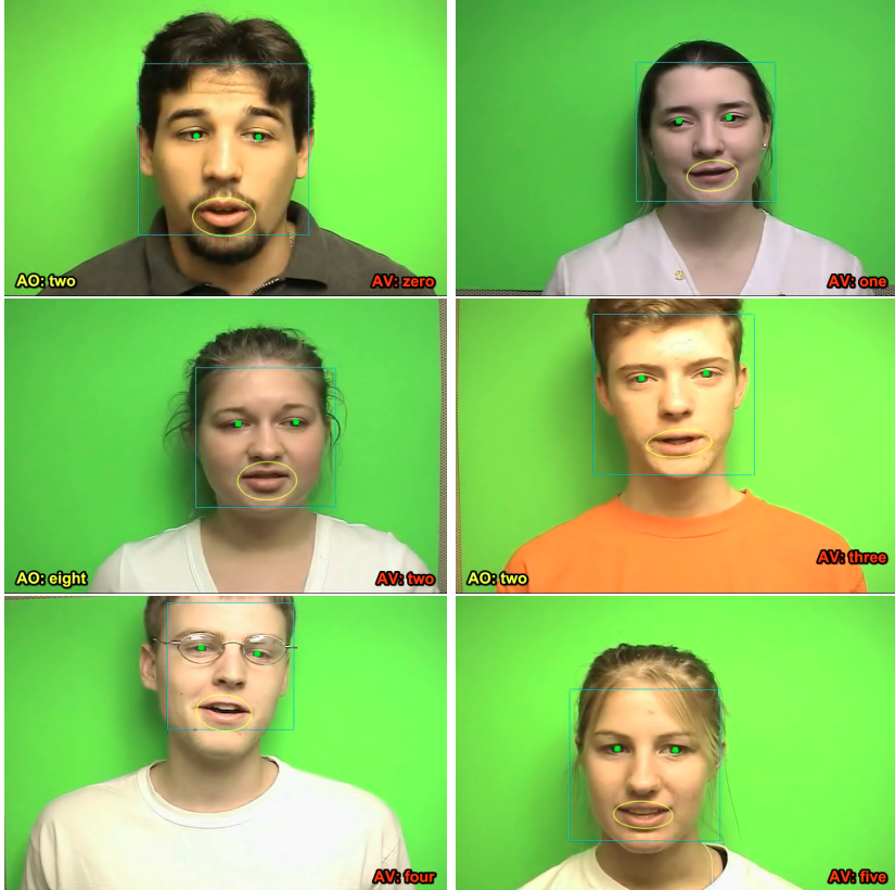
Figure 2.13: Some example frames showing the recognition capability of our system. The sequences were taken from the CUAVE database and white noise added to the audio channel (0 SNR). The yellow ellipse represents the localized mouth and the subtitles show the automatically recognized words. In these examples, the audio-visual system (AV - right) recognizes the word correctly, while the audio-only one (AO - left) makes mistakes or misses the utterance completely.
