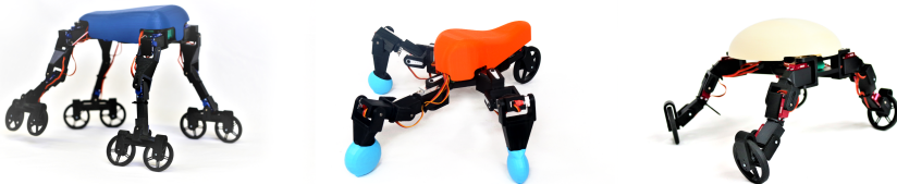
FIGURE 2.1: Robotic creatures created with our computational design system employ arbitrary arrangements of legs and wheels to locomote.
