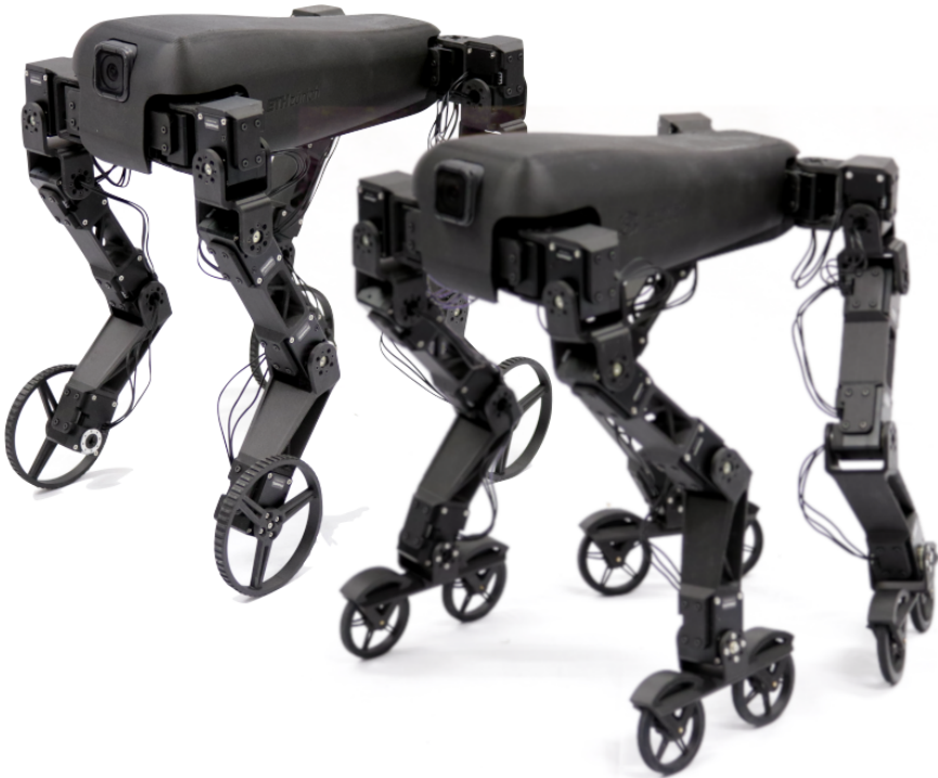
FIGURE 3.1: AgileBot and SkaterBot, two robots created with the help of our interactive design system.
