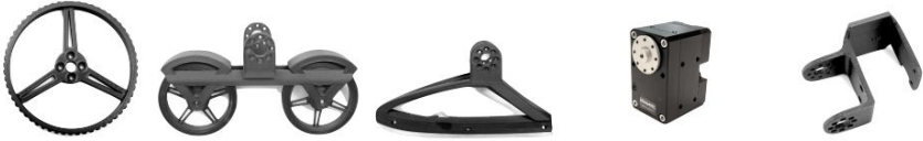
FIGURE 3.4: Our robots are made from 3d-printed parts and off-shelf electronic components for actuation and control. From left to right: 3D printed wheels that can be attached to a motor or left to spin freely, a roller blade with passive wheels and an ice skate, Dynamixel XM430-W210T are used to actuation joints and active wheels, and 3d-printed brackets.
