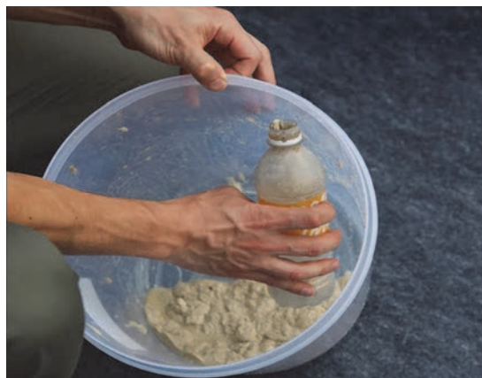
Figure 7.6 Faecal sludge simulant developed for prototype technologies at the Reinvent the Toilet Fair in India, 2014 ( www.mentalfloss.com/article/56003/recipe-fake-poop ).
