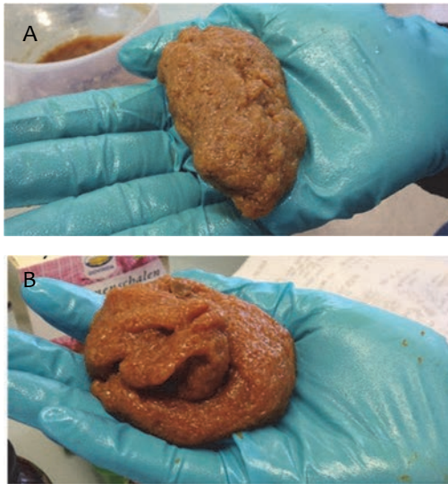
Figure 7.3 Simulants with 30 wt % of solids content yeast extract and no baker's yeast: A) SE65; B) SE80.
