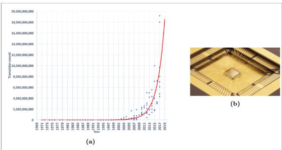
**Figure 1.** Technological progress. (a) number of transistors integrated on a single CMOS chip over the years (source 'the beauty and joy of computing—BJC'; (b) example of a recent neuromorphic CMOS VLSI chip comprising thousands of silicon neurons and dynamic synapses (source Institute of Neuroinformatics, University of Zurich and ETH Zurich).
