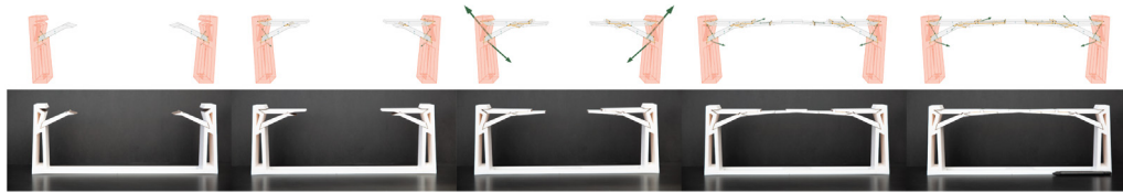
Fig. 15. Sequential scaffolding-free construction of the bridge. CRA analyses on top and corresponding construction phases on the small-scale physical models on the bottom.
