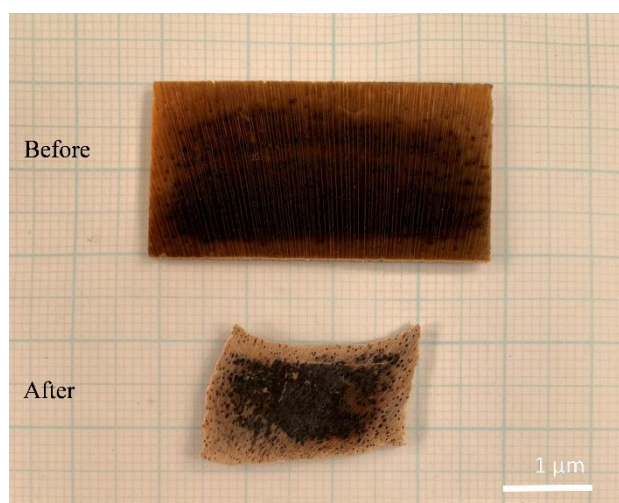
Figure S7. Photos of cross-cut balsa wood before and after ZIF-8 modification, showing the sample shrinkage.
