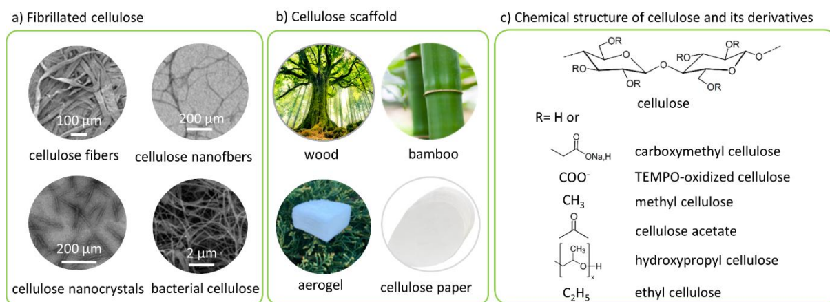
Figure 2 Examples of a) fibrillated cellulose including cellulose fibers, 51 cellulose nanofibers (CNFs), 52 cellulose nanocrystals, 51 and bacterial cellulose 53 and b) cellulose scaffolds including natural materials (wood and bamboo) and processed materials (aerogel 54 and cellulose paper) used for preparing MOF/cellulose composites. c) Chemical structure of cellulose and its derivatives
