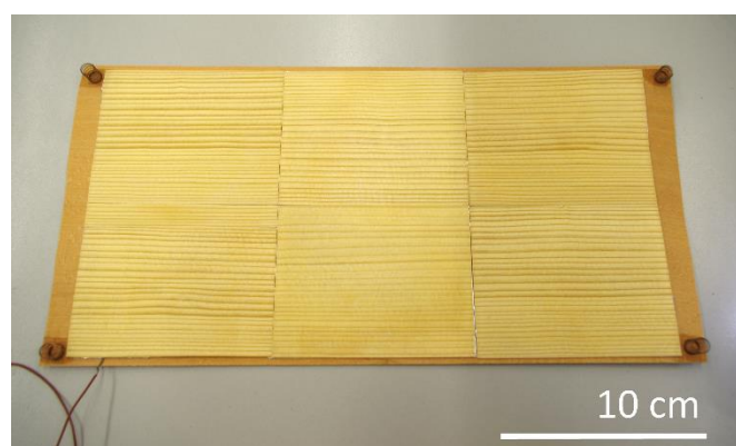
Figure S27. Photograph of a large-scale triboelectric wooden floor prototype (45 cm × 20 cm) made with six FW-TENGs electrically connected together.
