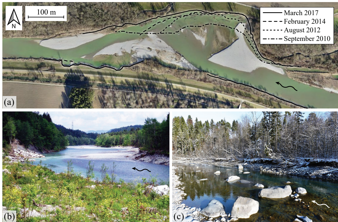
Figure 1.1 (a) Lateral erosion in the river widening Schaffäuli, Thur River (Orthophoto and data: geotopo ag, Frauenfeld), (b) pioneer vegetation in the river widening Augand, Kander River (Photo: Tiefbauamt des Kantons Bern, Oberingenieurkreis I, 2006) and (c) eroded riverbanks in the river widening Augand, Kander River. Both Thur and Kander River are gravel-bed rivers in Switzerland.
