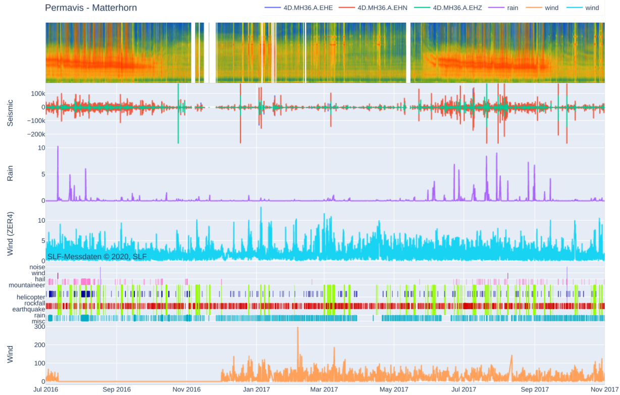
Figure 5.15 Joint visualization of seismic spectrogram, seismic waveform, rain and wind data of the Matterhorn deployment for a time period of more than a year . Additionally, the annotations of an event catalog and wind data from a nearby weather station (ZER4 by SLF) are plotted.
