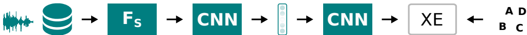
Figure 3.12 Data types, model and optimization used in this chapter. Machine learning-based information extraction from waveform data (seismic and audio) using a data specific frontend ( F_W ) and convolutional neural networks (CNN) optimized with cross-entropy loss (XE) using a set of labels.
