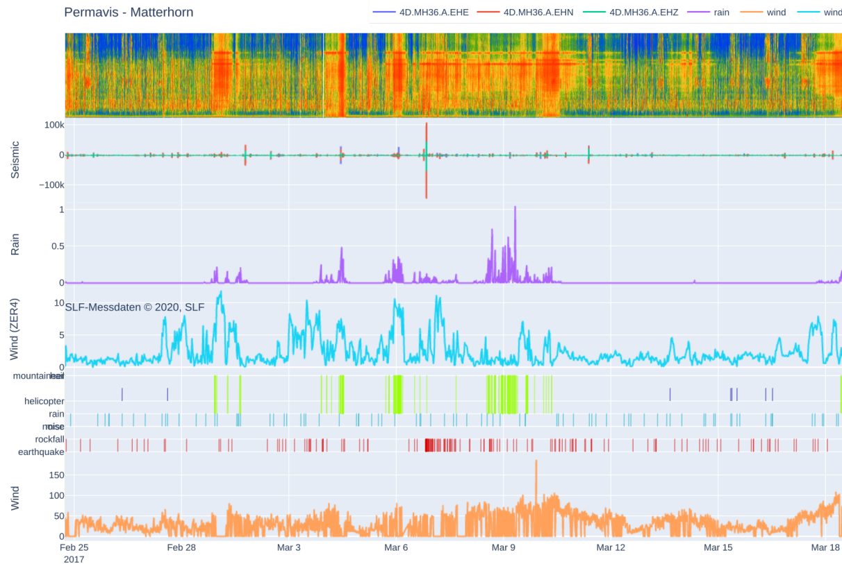
Figure 5.16 Joint visualization of seismic spectrogram, seismic waveform, rain and wind data of the Matterhorn deployment for a time period of multiple days . Additionally, the annotations of an event catalog and wind data from a nearby weather station (ZER4 by SLF) are plotted.
