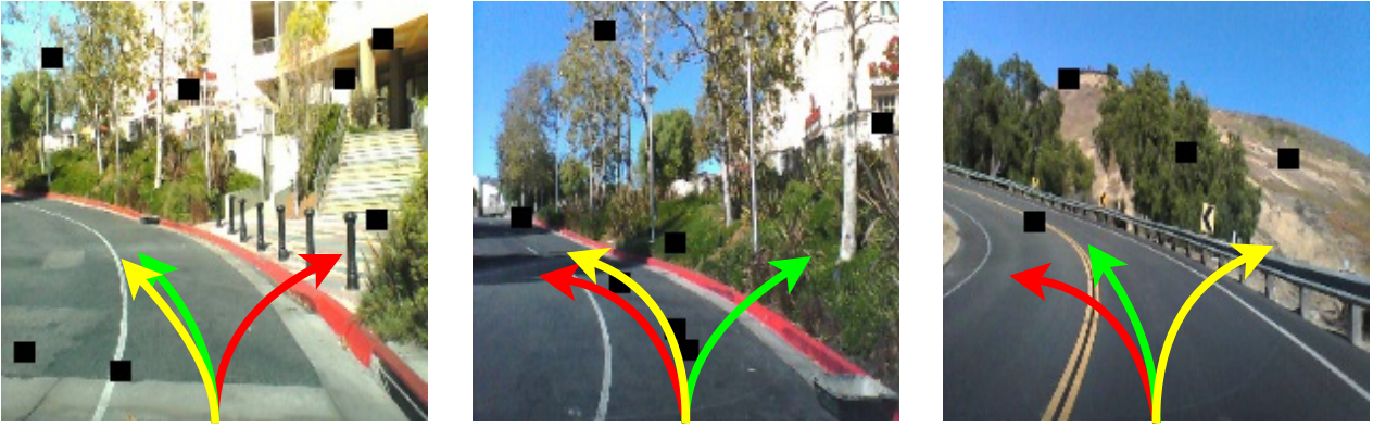
(a) Black rectangle defects in natural images. Each image fools one of three different classifiers [131].
