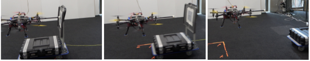
(a) The aerial vehicle regulates a pushing force on the cart. (b) The cart is pulled away and the platform loses contact. (c) The force dynamics divergence is detected and the platform stops without diverging.
