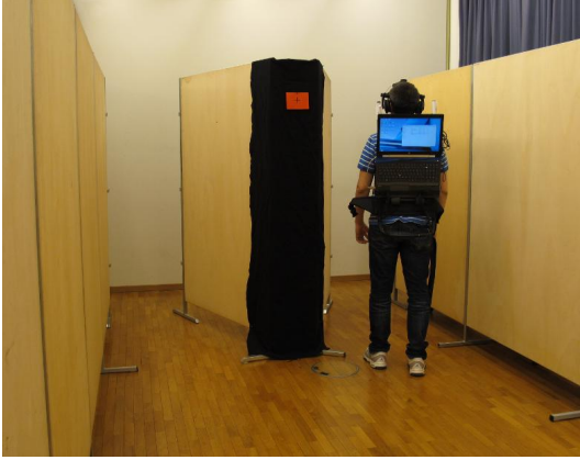
Figure 2. Picture of the study setup. A subject wears the backpack with the notebook and the HMD with the tracking system. The red paper in the middle is the center mark for the initial calibration.
