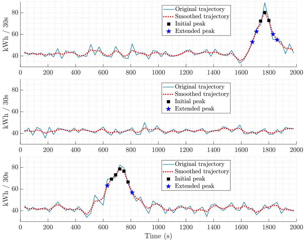
**Figure 1:** Examples of simulated system energy trajectories and detected peaks.
