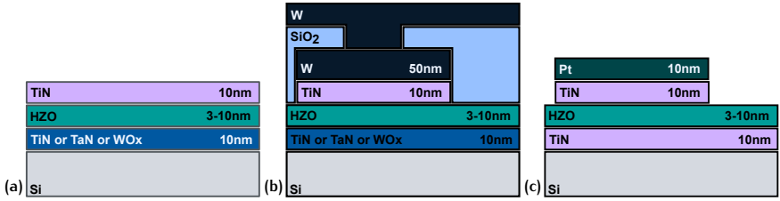
Figure 4.6: Schematic representation of structures used to analyse different bottom electrodes: (a) For GIXRD, (b) for PUND, and (c) for PFM.
