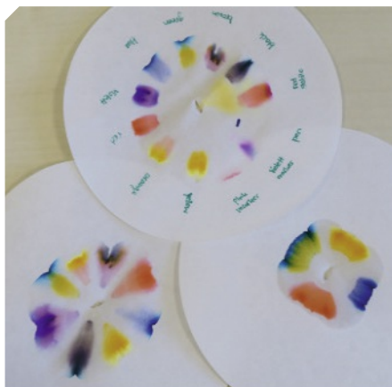
Fig. 2. Examples of paper chromatography with colorful pens.
