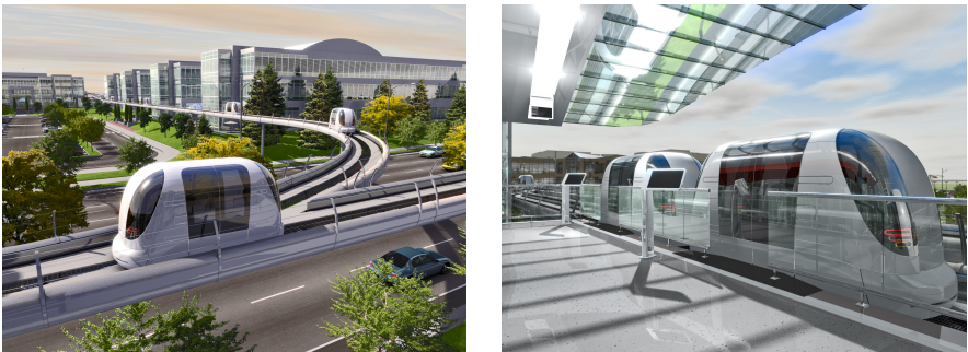
Figure 5.1: Visualizations of Personal Rapid Transit. Left: Track junction with pods. Right: PRT station. Both renderings are reproduced here by courtesy of Ultra [ULT11].
