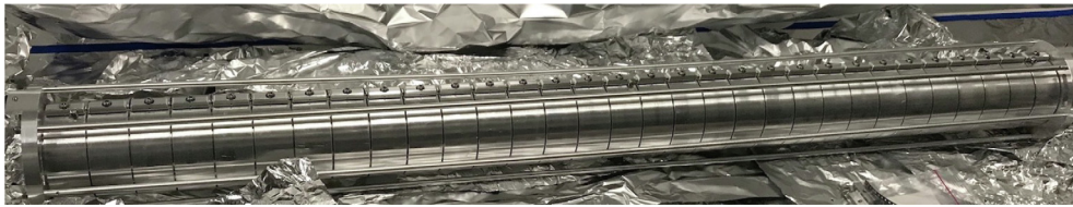
Fig. 3. The electron repeller consisting of 31 electrodes.
