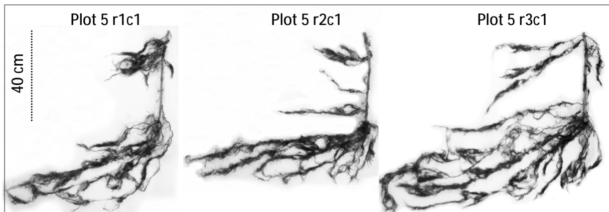
Figure E.1: Black and White pictures of the three samples taken from plot 5 in September 2009. The three pictures are then separately analyzed using the Matlab software. Input parameter for analysis are specified by means of the user's interface of shown in figure E.2.
