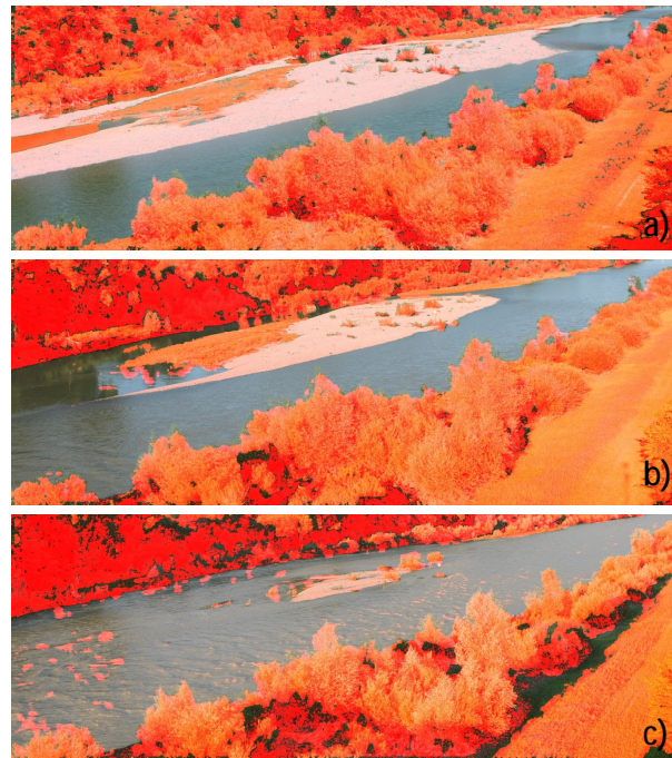
Figure 2.8: The automatic algorithm for pattern recognition allows delimitation of water and non-water classes from digital photographs. The reddish mask over the pictures represents the pixels classified as non-water.
