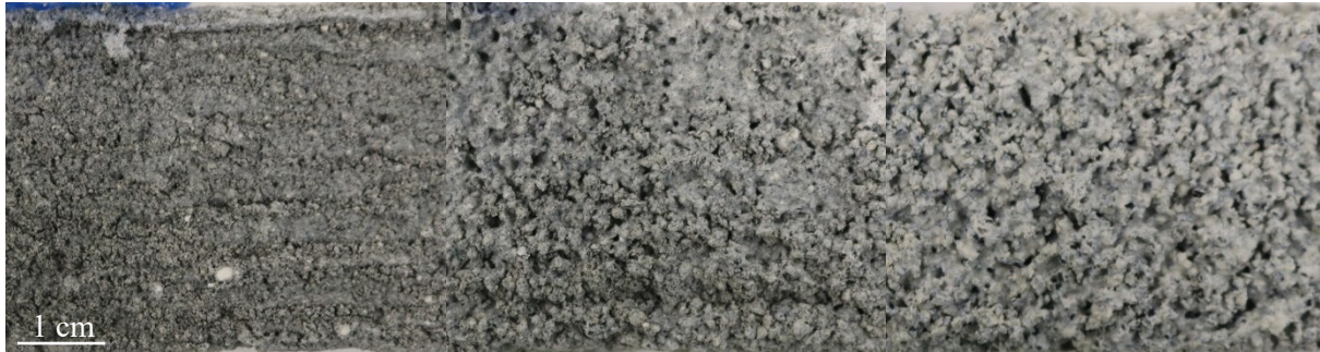
Figure 12: Texture (side view) of prints on fine (left), mix (middle), and coarse (right) Bettazza grains
