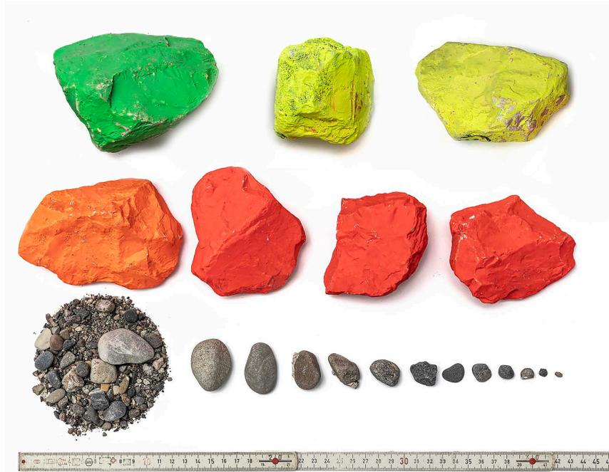
**Figure 4.12** Step-forming blocks (coloured) used for the artificial step-pool sequences and sediment mixture SM64 (model scale [cm])
