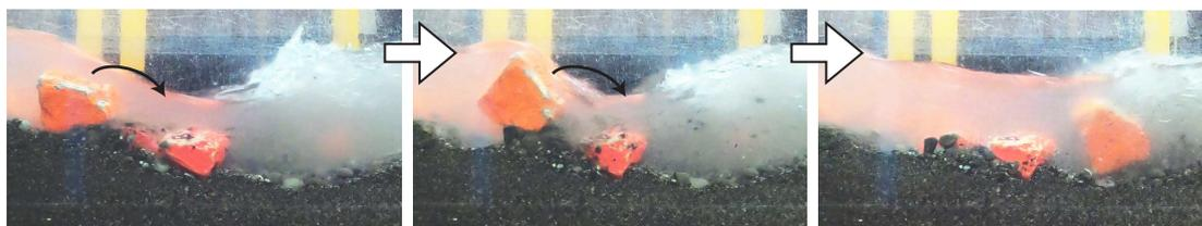
**Figure 4.17** Monitoring of failure mechanisms showing frames extracted from a time lapse video recorded with a GoPro 8 through the glass sidewall of the flume ( $\Delta t \approx 2.2$  s in between photos in prototype scale)
