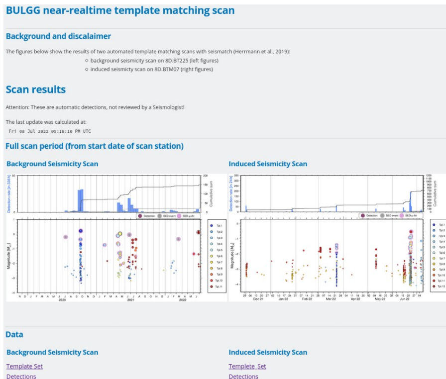
Fig. 7) Screen shot of the internal webpage displaying the results of two template matching scans for the BedrettoLab.
